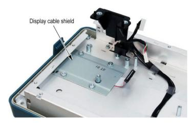
Figure 4-5: Display cable shield in place
