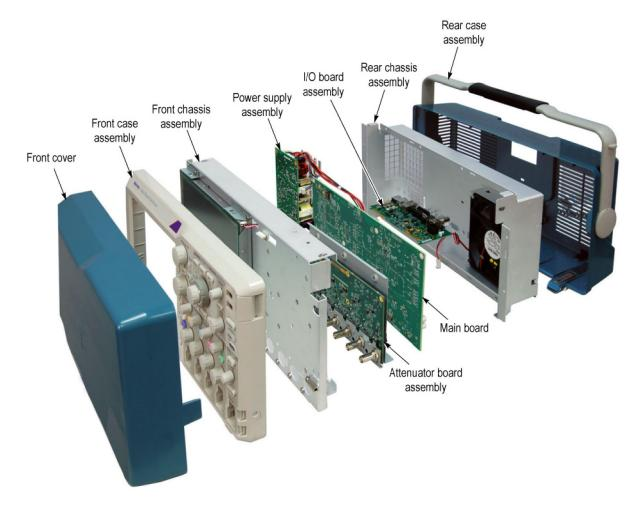
Figure 4-1: Locator for internal modules
