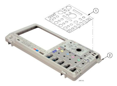
Figure 5-4: Exploded view: Front panel labels
