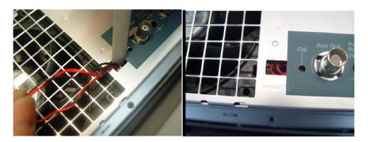
Figure 4-2: Reconnecting the fan cable
