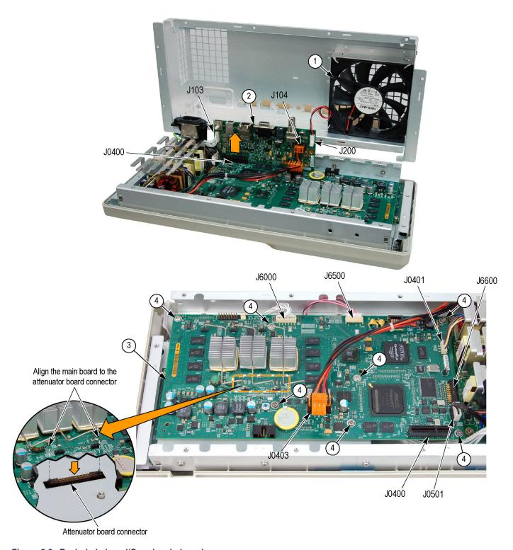
Figure 5-2: Exploded view: I/O and main boards
