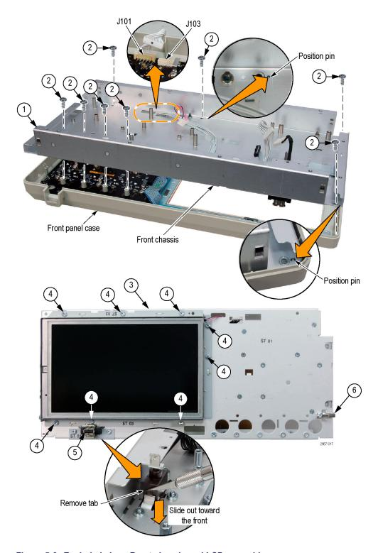
Figure 5-6: Exploded view: Front chassis and LCD assembly
