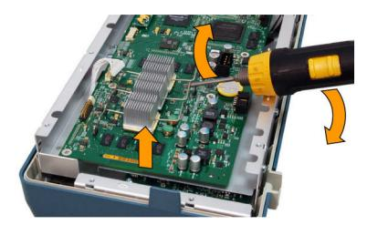
Figure 4-4: Disconnecting the main board
