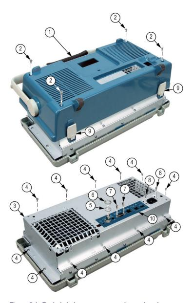
Figure 5-1: Exploded view: rear case and rear chassis
