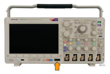
Figure 3-5: Digital channel input (MSO only)
