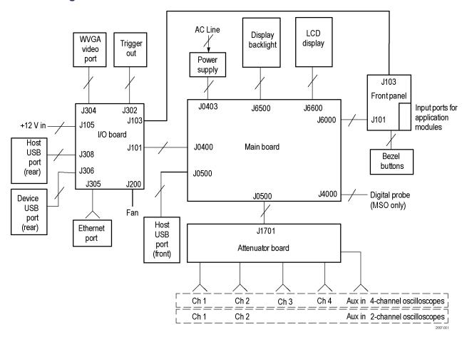
Figure 2-1: Oscilloscope module interconnections
