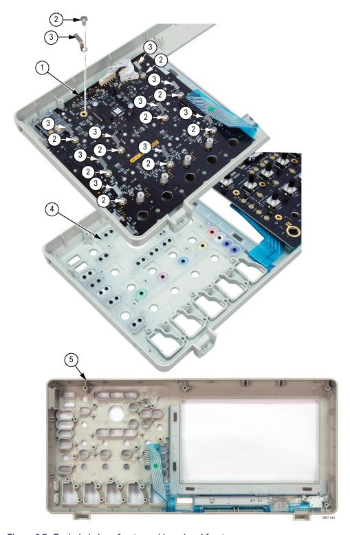
Figure 5-7: Exploded view: front panel board and front case
